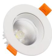
Specifications LED Spot Round Tilttable 9W 720lm - 840 Cool White | 108mm - Cutout 90mm - UGR<19
